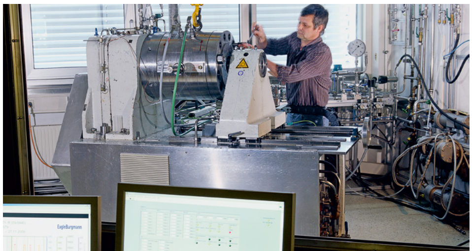
One of the test rigs for running seal qualification tests according to API at EagleBurgmann.
