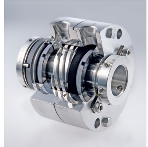
EagleBurgmann mechanical seal type LL9DTUU (API seal type A, rotating).
